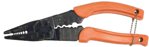
20716 Multi-Function Crimping Tool Cuts/Strips/Crimps 22-10 ga. Non and Insulated Terminals, Flag Terminals, Bolts, W/ Pliar Tip and Spring Loaded Handle Length 8-5/8"
